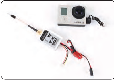
1.1 Prepare GoPro camera(please purchase it separately and connect the video cable in advance) and 5.8G(TX5803/TX5804) emitter.
