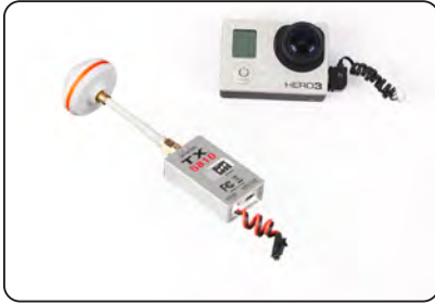
3.1 Prepare GoPro camera (please purchase it separately and connect the video cable in advance) and 5.8G(TX5810/TX5811) emitter.
