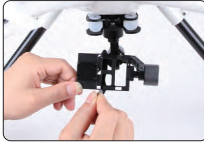
1.2 Unscrew two M2x4 screw, Loosen the camera fixed frame.
