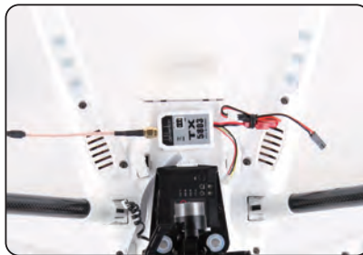
1.5 Install the 5.8G(TX5803/TX5804) emitter to the copter bottom with double side tape.
