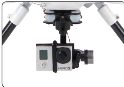
3.8 Camera and 5.8G(TX5810/TX5811) emitter installation finished (make sure the camera cable is free so the camera can move freely).
