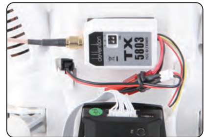
1.6 Insert the emitter power cable into power output port(DC 12V) of copter.
