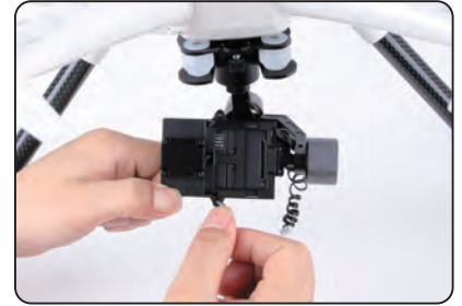
3.3 Install the camera into gimbal, Fix it with camera fixed frame (ensure the gap close to the lens), then screw the M2x4 screw to the camera fixed frame again.
