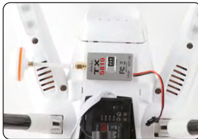
3.5 Install the 5.8G(TX5810/TX5811) emitter to the copter bottom with double side tape.
