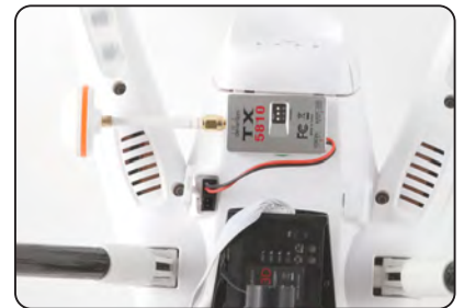
3.6 Insert the emitter power cable into power output port (DC 12V) of copter.
