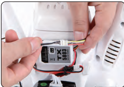
1.7 Connect the Gopro video cable with the image signal cable of (TX5803/TX5804) emitter.
